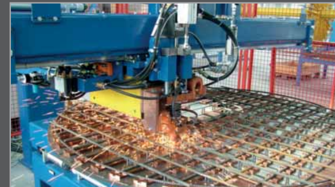
Special machine type GSM for welding of mats for manhole bases
