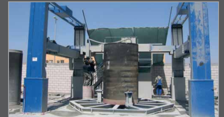
Special machine type VFM for vertical milling of concrete pipes
